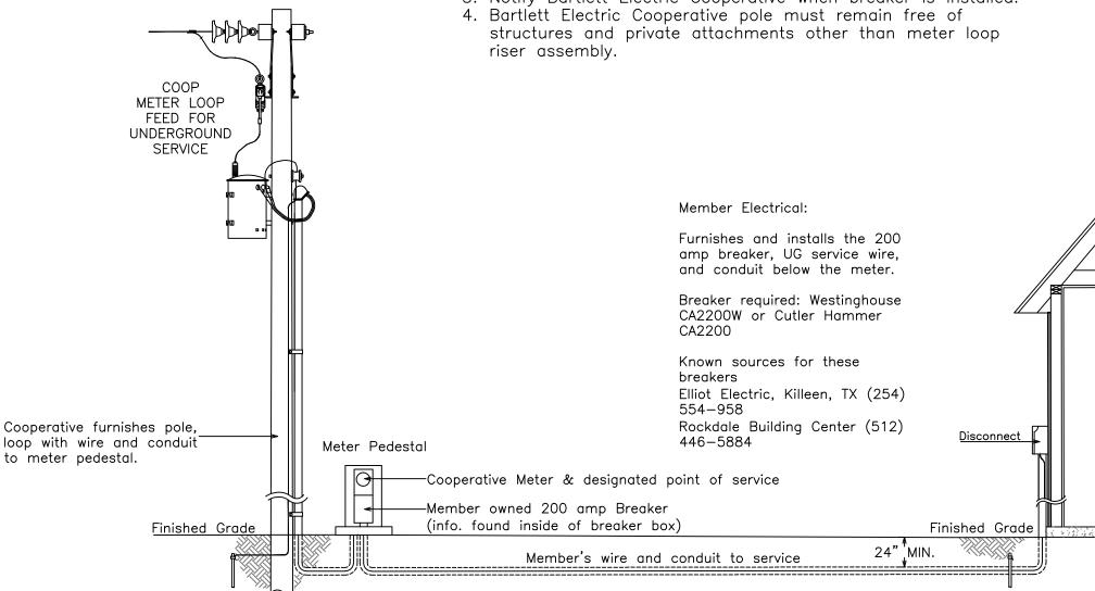
FOR THE MEMBER'S SAFETY, WIRING INSTALLATIONS SHALL CONFORM TO THE REQUIREMENTS OF THE NEC AND NESC.
